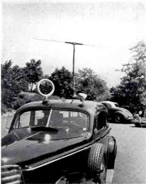
FIG. 12. The equipment shown in Figure 11 is mounted in this field car, one of several belonging to the NBC Allocations Staff. Dipole antenna projects from the roof of the car.
