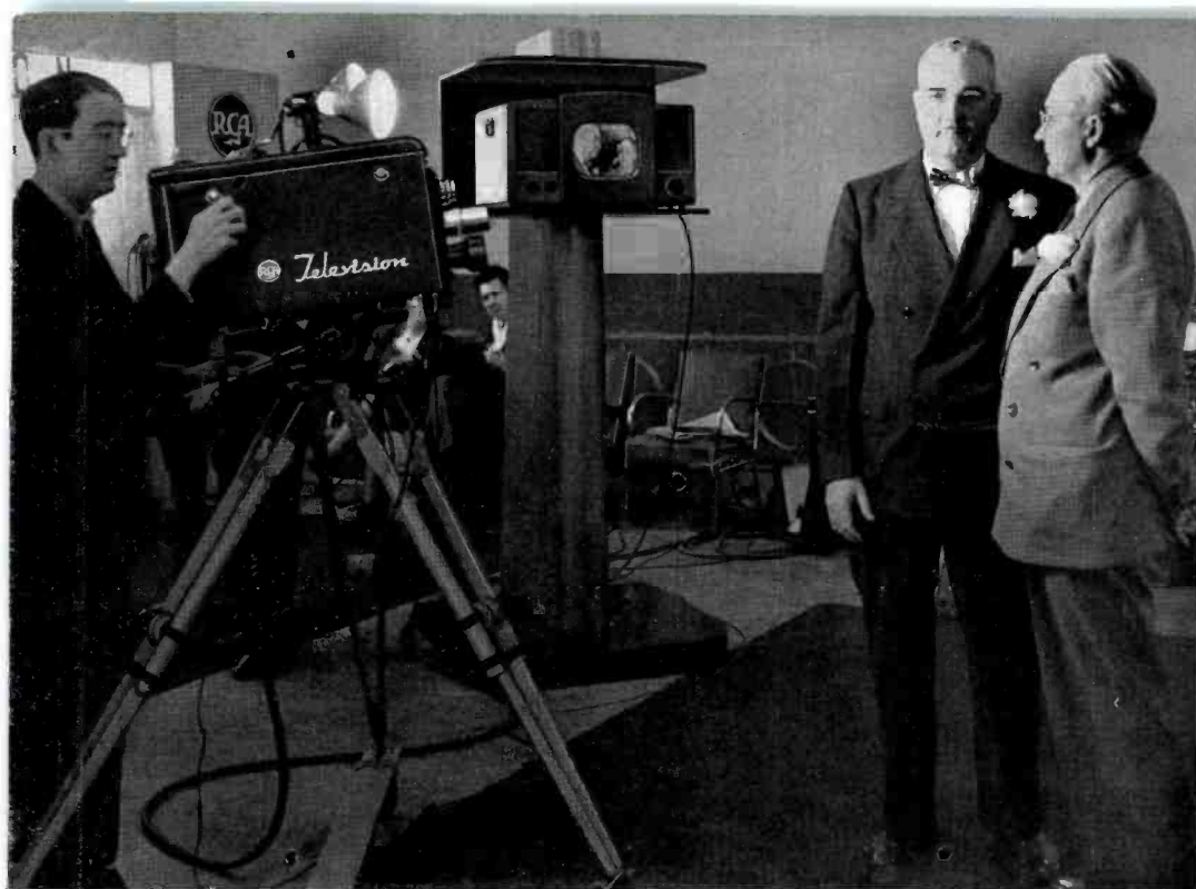
FIG. 1. (Left)—“Seeing themselves in television” has been the unusual experience of thousands of persons throughout the country during television demonstrations by RCA. The receiver shown here is a standard television receiver (Model 630 TS) modified for use as a video extension monitor. The coaxial cable input to the receiver can be seen just below the receiver in the photo.
