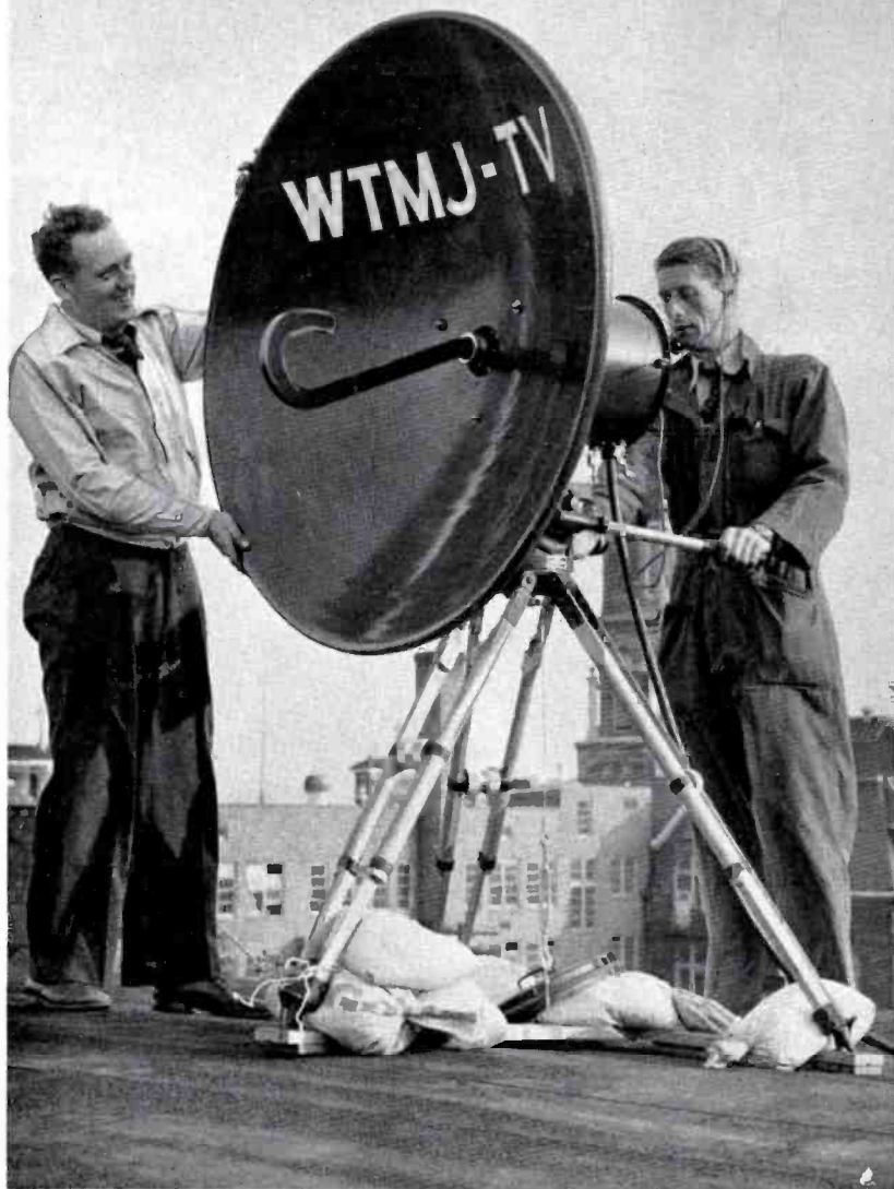
FIG. 1. WTMJ-TV's new television equipment includes complete RCA Microwave Equipment for relaying remote programs to the studio.
