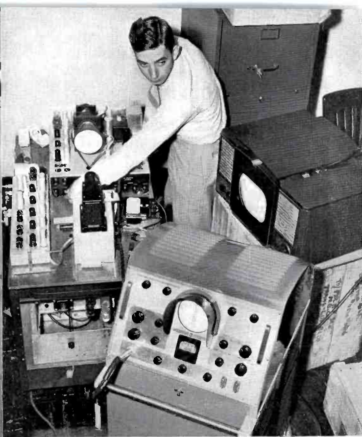
FIG. 7. Lining up the flying spot generator built by NBC engineers for use in generating test patterns.
