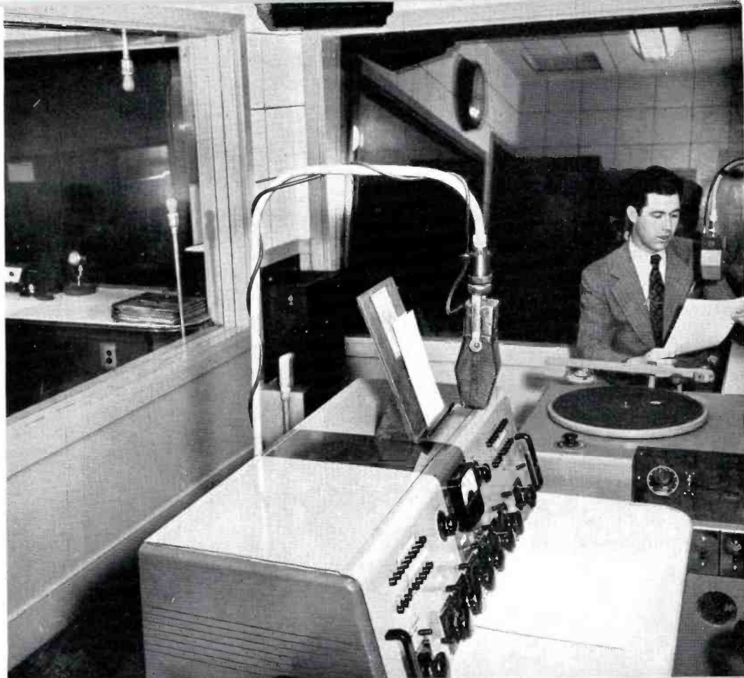
FIG. 3. Studio control booth and announce position at KFBK. In the foreground is an RCA 76-B2 Console with a 44-BX microphone suspended over it. At the right of the console are two 70-B Turntables built into a convenient dual housing. Announcer sits at 74-B microphone just beyond turntables. Window at left looks into master control room (a partial view of which is shown on the opposite page). Window at rear looks into large studio.
