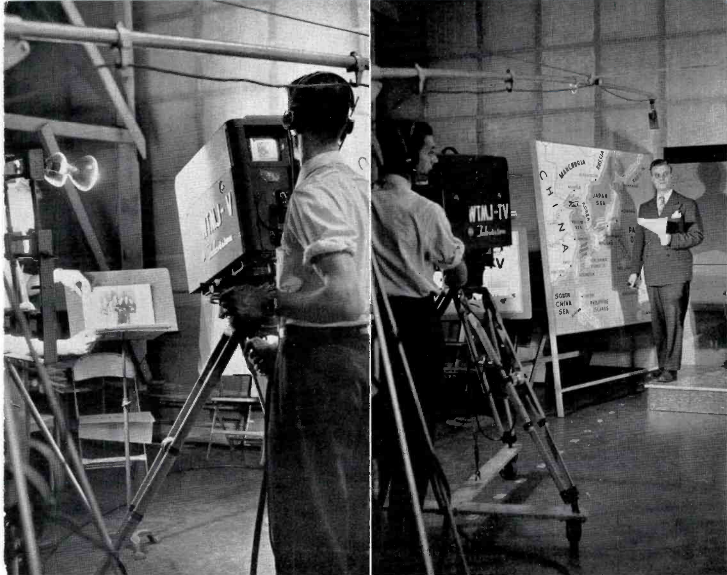
FIG. 2. Two image-orthicon field camera chains are included in WTMJ-TV's equipment. At present these are used for both studio and field use. Additional cameras which have been ordered will be installed for permanent studio use.
