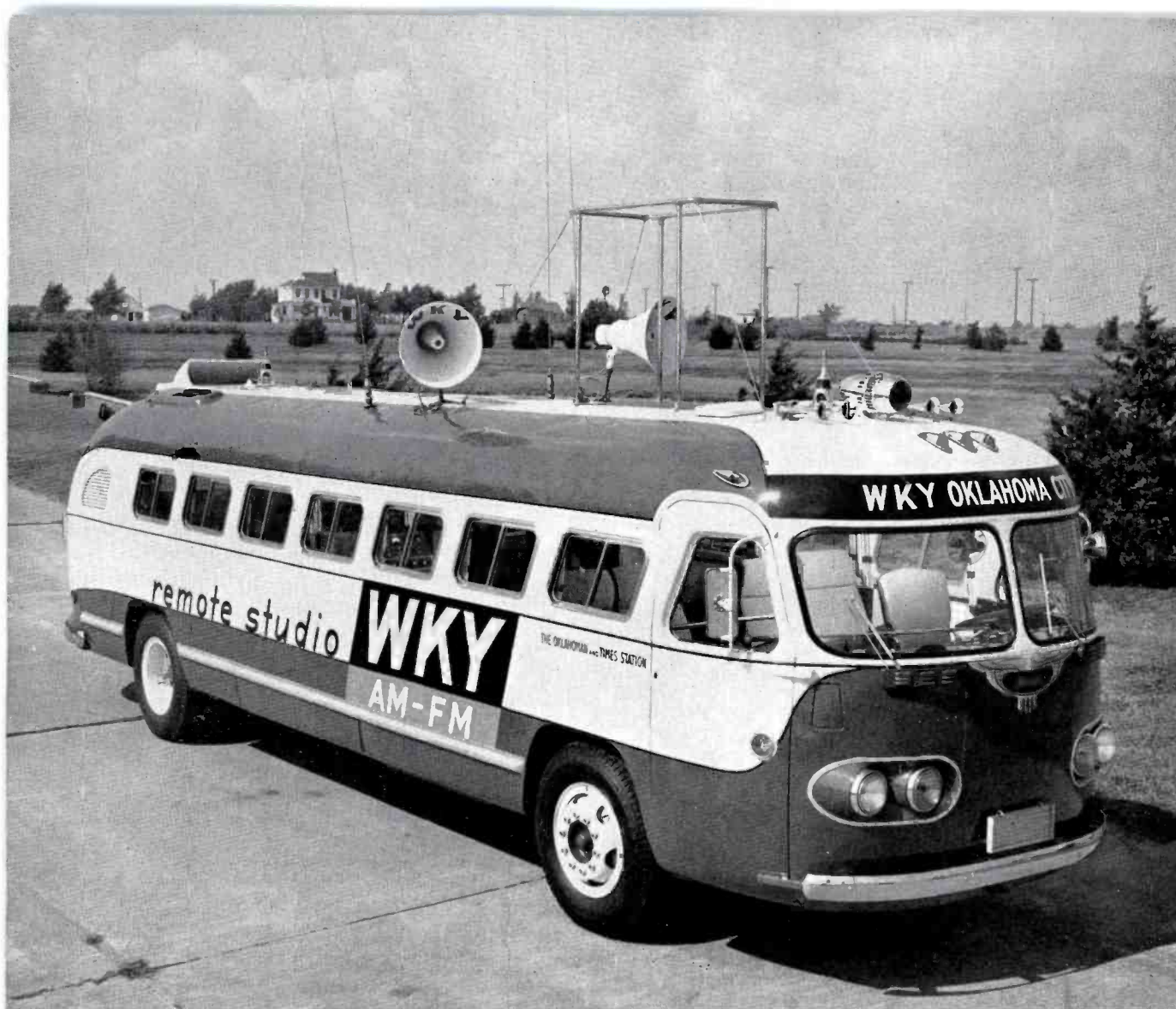
FIG. 1. WKY's mobile unit—built to permit coverage of an entire state—is a 29 passenger bus body, custom-converted by the bus manufacturer according to plans drawn by WKY's engineering staff. Complete facilities and comfort for traveling are outstanding features.
