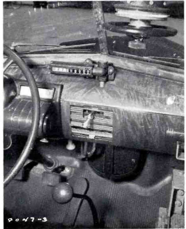
FIG. 13. In order to coordinate recorder readings with the location of the car, the recorder chart mechanism is geared to the speedometer drive shaft. Clutch is shown in this view.
