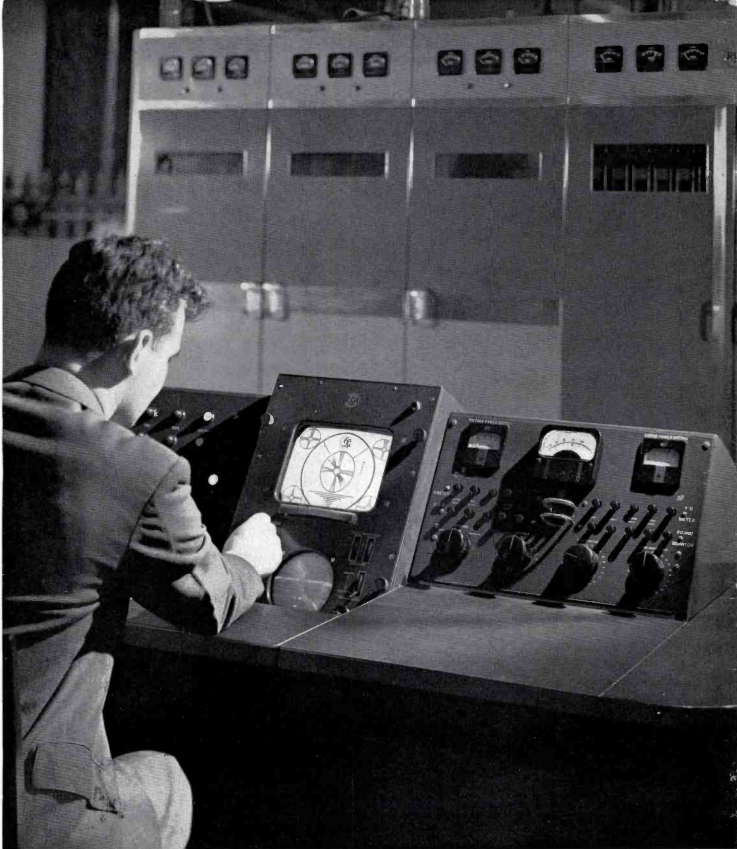
FIG. 16. The control console furnished with the TT-5A is one of the outstanding features of this transmitter. From this vantage point the operator has complete finger-tip control over both the operating and monitoring functions of the transmitter. In the center of the console is a standard RCA TM-5A Monitor containing a 10-inch picture tube, for observing the transmitted picture, and a 5-inch CR tube, for monitoring the wave form. Both may be switched to the incoming line for checking purposes. At the sides of the monitor unit are two sloped panels (on opposite page) containing all of the usual transmitter starting and operating controls.
