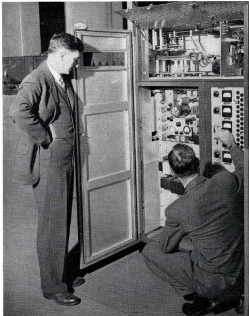
FIG. 10. (right) Open view of frames 1 and 2 containing the sound transmitter. The lower part of frame 1 (left) contains a standard RCA FM exciter unit. The lower part of frame 2 (right) contains the intermediate stages, while the power amplifier is arranged horizontally across the top part of the two frames. In this illustration H. E. Gihring (right), manager of RCA Television Transmitter Engineering Section, explains operation of sound transmitter to Henry Rhea, formerly manager of RCA Television Equipment Sales, now manager of WOWH, Clinton, Illinois.
